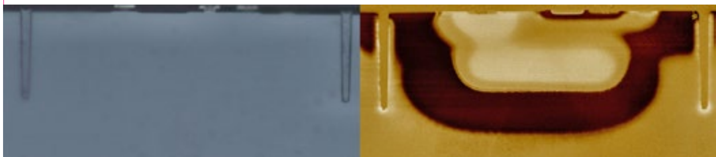
Figure 3: SCM image showing a cross-section of a PNP bipolar transistor.
